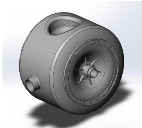
Figure 5: Schematic of Spoke040 cavity and stiff ribs.
