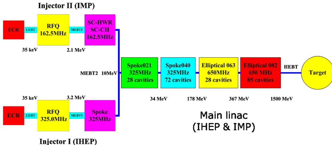
Figure 1: Layout of ADS accelerator.
