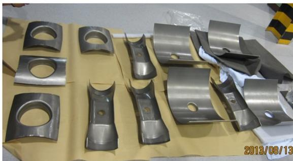
Figure 7: Components after deep-drawing.
