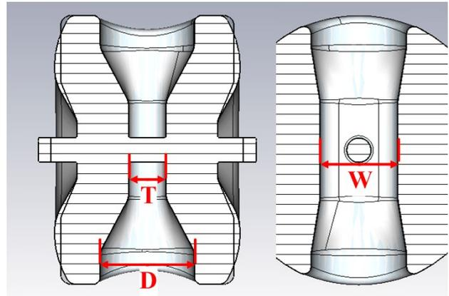
Figure 2: Flat and convex end-wall of Spoke040.
