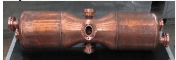
Figure 4: HWR copper model.
