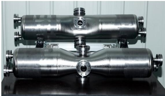
Figure 7: The fabricated HWR010.
