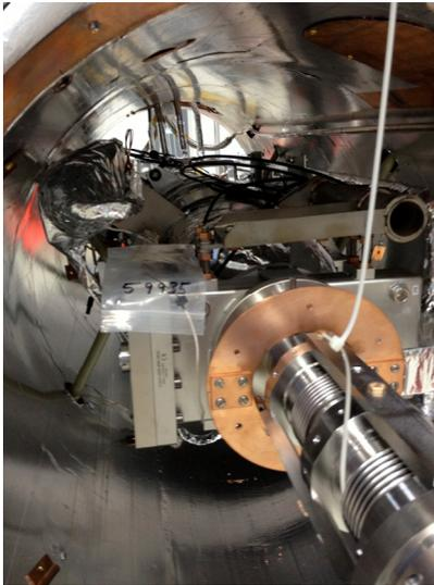
Figure 4: CC-1 internal view with new cavity inserted.
