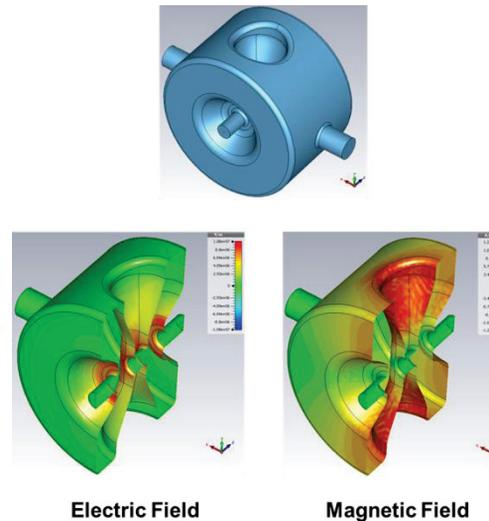
Figure 1: SSR1 cavity having flat end walls and its field distribution.
