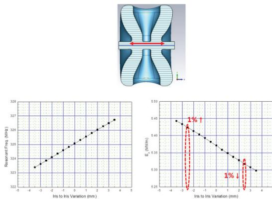
Figure 3: Variations of resonant frequency and longitudinal electric field with respect to iris-to-iris distance in the SSR1 cavity.
