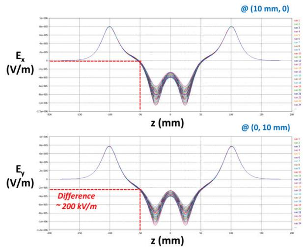
Figure 4: Variations of transverse electric fields along longitudinal axis with different elliptical beam tunnels at the spoke.
