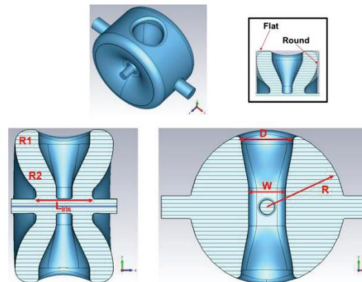
Figure 2: SSR1 cavity having rounded end walls.
