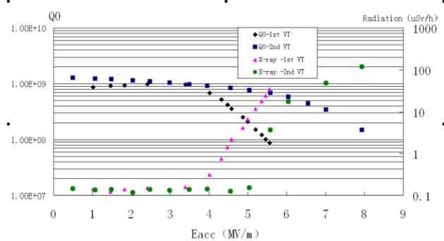
Figure 5: Results of vertical testing of spoke012-2.
