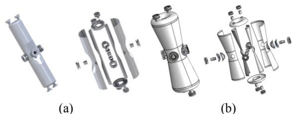
Figure 9: Structures of HWR010 (a) and HWR015 (b).
