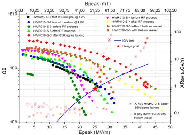
Figure 10: Vertical testing results of HWR010-02~05.
