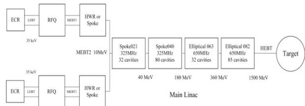
Figure 2: Conceptual design of accelerator for China ADS project.
