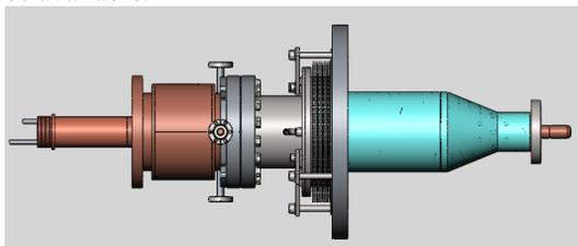
Figure11: General layout of coupler for HWR.
