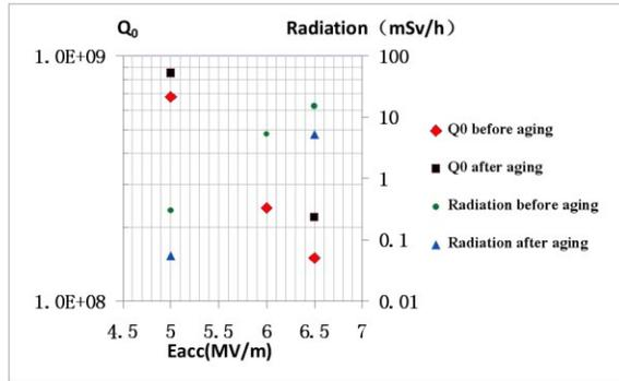
Figure 6: Results of horizontal testing of spoke12-2.
