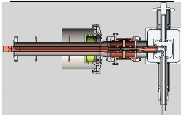
Figure 7: Cross-section view of coupler.
