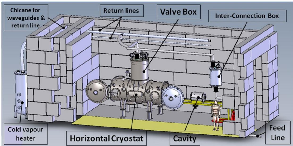
Figure 1: Layout of the FREIA bunker.
