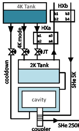
Figure 2: Valve Box Flow diagram.
