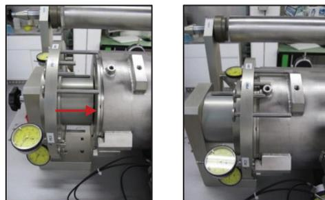
Figure 2 and 3: Wheel with dial gauges and gauging jigs.
