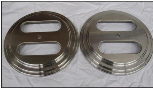
Figure 4: Gauges for checking diameters of bellow unit, reduction ring and sliding collar.
