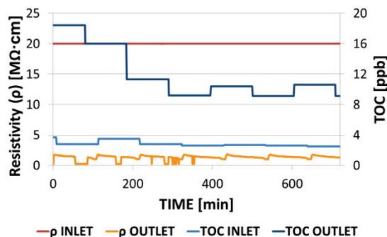
Figure 4: HPR recording with resistivity ( $\rho$ ) and TOC.
