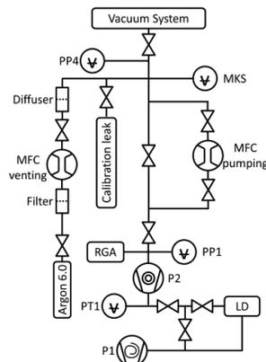
Figure 2: SPSV layout. With reference to the above: PP1 and PP4 are UHV gauges, PT1 is a Pirani gauge and MKS is a differential gauge.
