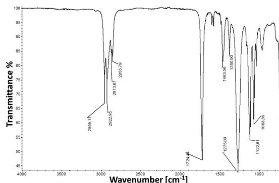
Figure 5: FTIR spectra of DEHP found in ethanol.
