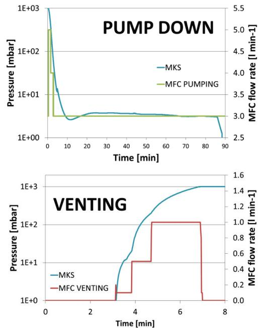
Figure 3: SPSV pressure and flow rate (10<sup>3</sup>-1 mbar).
