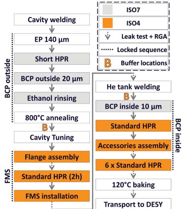
Figure 1: EXFEL Cavity treatment cycle.
