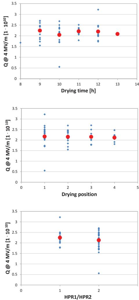
Figure 6: Influence of the last operations in ISO4 (drying and HPR) on the series cavity performances (Q). Q @ 4 MV/m measured for each cavities (blue), average value (red).
