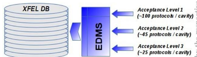
Figure 2: Cavity production dataflow.
