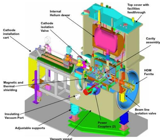
Figure 1: Layout of the 704 MHz ERL gun cryomodule.
