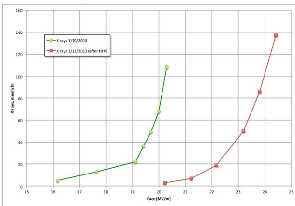
Figure 2: X-ray level near the SRF gun before and after high-power RF processing.
