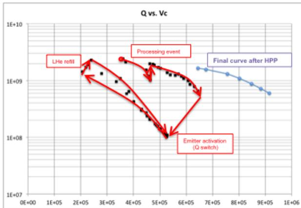
Figure 4:  $Q$  vs.  $V_c$  plot showing the gun cavity behavior during conditioning and the final curve.
