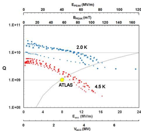
Figure 15: Plots of 5 QWRs tested for ATLAS upgrade (Courtesy of ANL).
