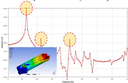
Figure 5: Analysis of mechanical vibration modes and characteristic frequencies of QWR cavity with He jacket. Lowest mode frequency is 160 Hz and the next 280 Hz.
