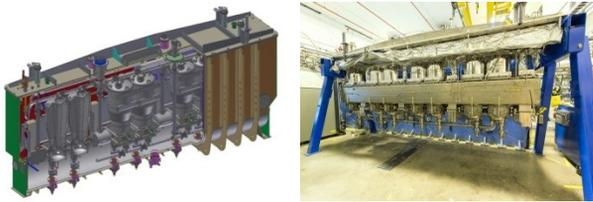
Figure 14: ATLAS upgrade cryomodule drawing on the left and photograph of cryomodule assembly on the right (Courtesy of ANL).
