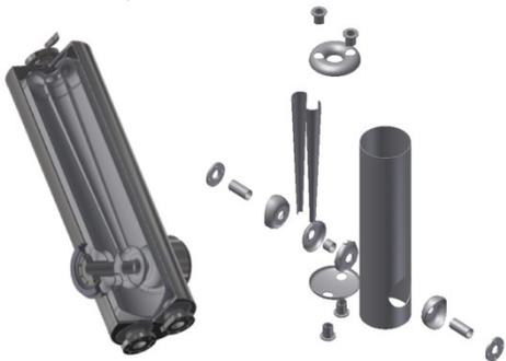
Figure 6: Drawing of QWR with helium jacket.
