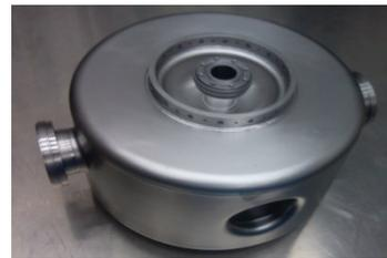
Figure 13: The spoke021 cavities parts (Courtesy of IHEP).
