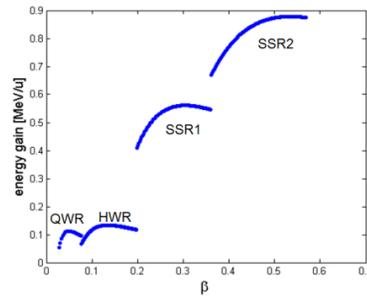
Figure 3: Plots of the optimized geometric betas of the superconducting cavities of RAON SCL.
