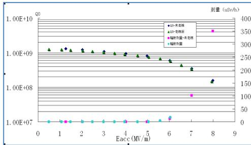
Figure 10: Vertical test result of Spoke012:  $Q_0 = 5.8 \times 10^8$  @ 6MV/m, 4K;  $Q_0 = 3.4 \times 10^8$  @ 7MV/m, 4K (Courtesy of IHEP).
