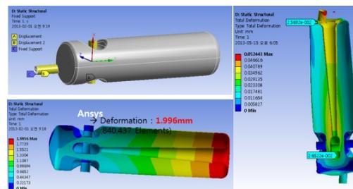
Figure 4: Plot showing thermal contraction due to cool-down to 2K and stiffeners reduces frequency shift by cool-down and pressure change.
