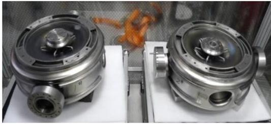
Figure 9: Two fabricated spoke012 prototype cavities (Courtesy of IHEP).
