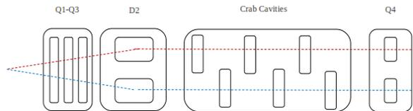
Figure 3: Schematic of the crab cavity layout on each side of the IP (not to scale).
