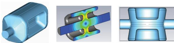
Figure 4: Three potential compact cavities under study for the HL-LHC upgrade [3–5].
