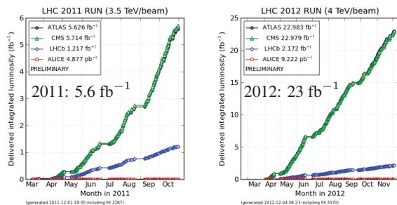
Figure 1: Integrated luminosity delivered to each of the four experiments in the LHC in 2011 (left) and 2012 (right), (courtesy LHC-OP).
