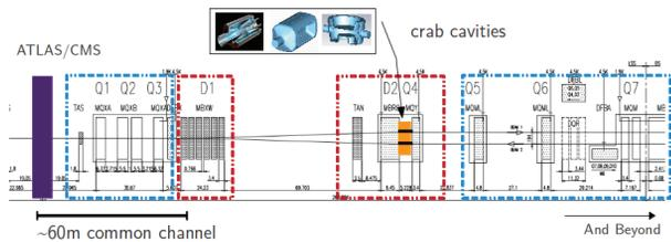
Figure 2: Schematic of the LHC interaction region and the respective magnetic elements to be upgraded with the inclusion of crab cavities for HL-LHC.
