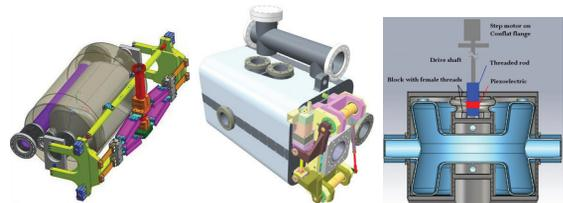
Figure 8: Dressed cavity concepts with their tuning assemblies [13].
