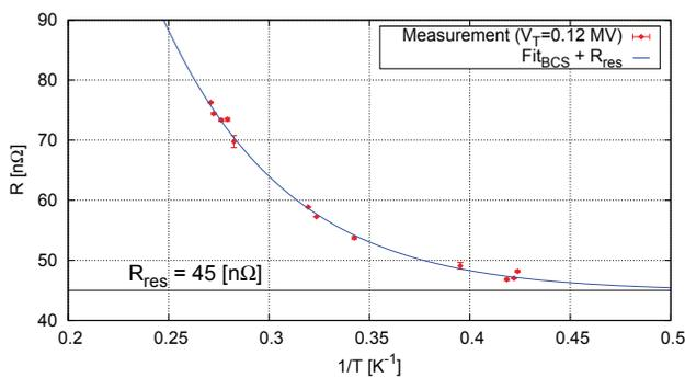
Figure 7:  $R_s$  vs. temperature at a fixed  $V_T = 0.12$  MV (Courtesy BE-RF).
