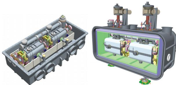
Figure 9: A top loaded and side loaded concept for the two-cavity SPS test module [14].
