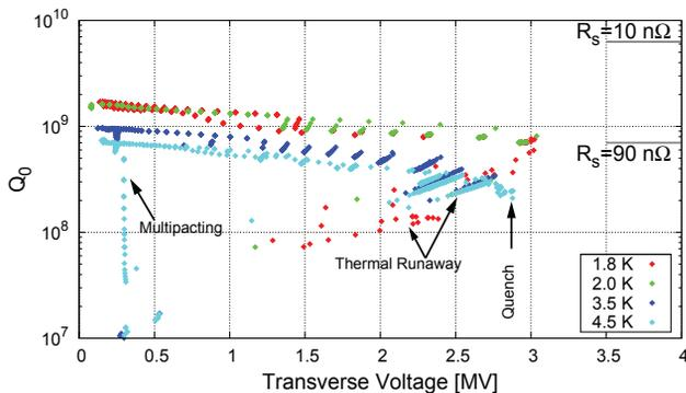
Figure 6: Second test results after light chemistry from 4.5K down to 1.8K (Courtesy BE-RF).
