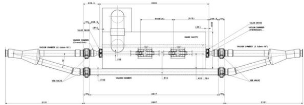
Figure 5: The SPS-BA4 region with a horizontal bypass which is the planned location for a crab cavity test module.
