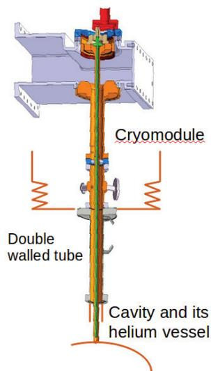
Figure 10: Standardized power coupler assembly with a single co-axial disk ceramic.
