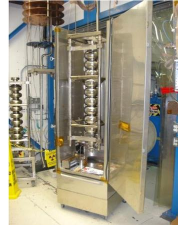
**Field flatness check, Ultrasonic, flash BCP, HPR, Assemble, Baking at JLAB**
