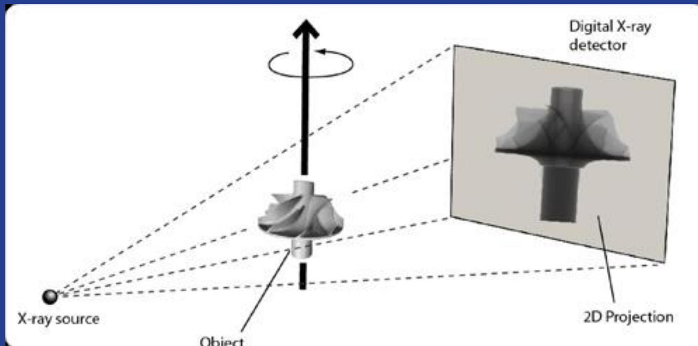
The X-ray tube (open or sealed) produces a conic beam of electron that penetrates the object to be analyzed, and a digital signal is interpreted by the 2D detector as a Digital Radiograph image.
