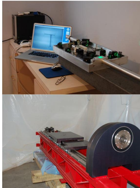
Microdynamics internal optical inspection system will be commissioned in this August. Enable detailed analysis of surface evolution as a function of EP parameters applied to single /multi-cell cavities.
