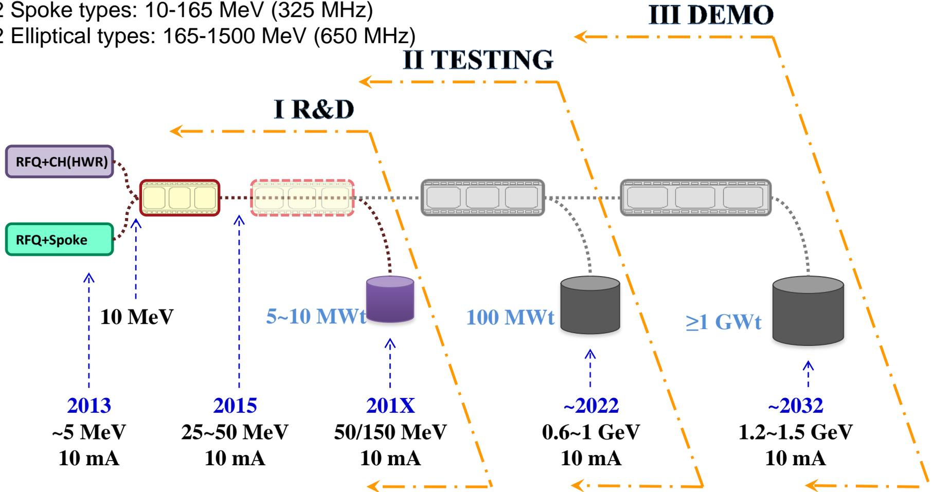
C-ADS is being developed by CAS. IHEP and IMP are in charge of proton accelerator. The facility is dedicate for transmutation and subcritical reactor. The project will be three stages. It is for technology R&D in the first 5 ~ 7 years.
