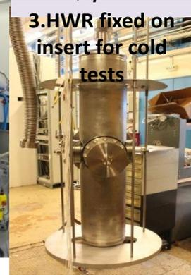
3.HWR fixed on insert for cold tests
