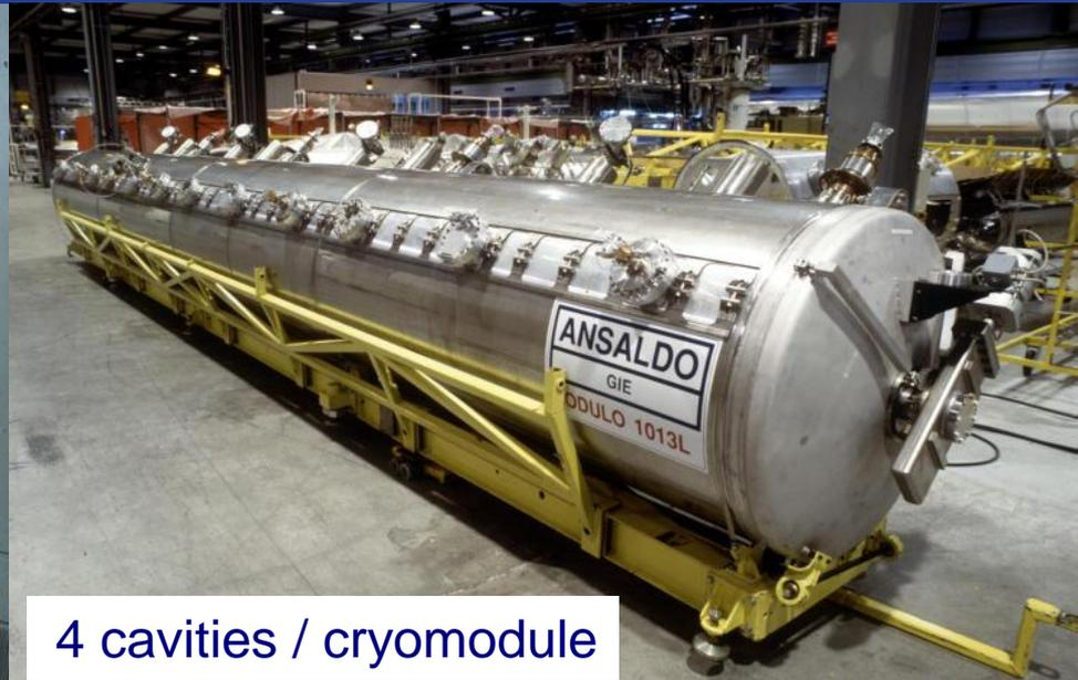
4 cavities / cryomodule
