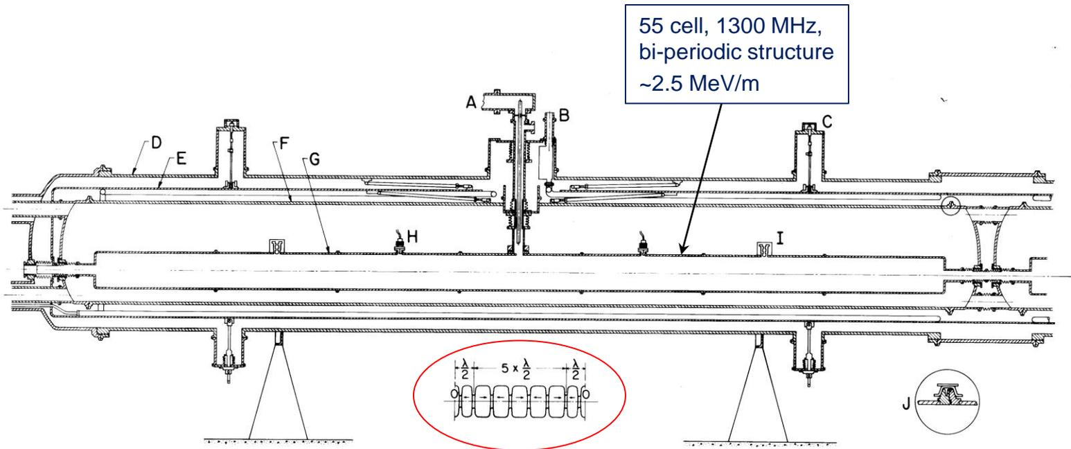
Assembled 20-foot accelerator dewar module. This section has end caps at one end and is connected to another module at the other end.
