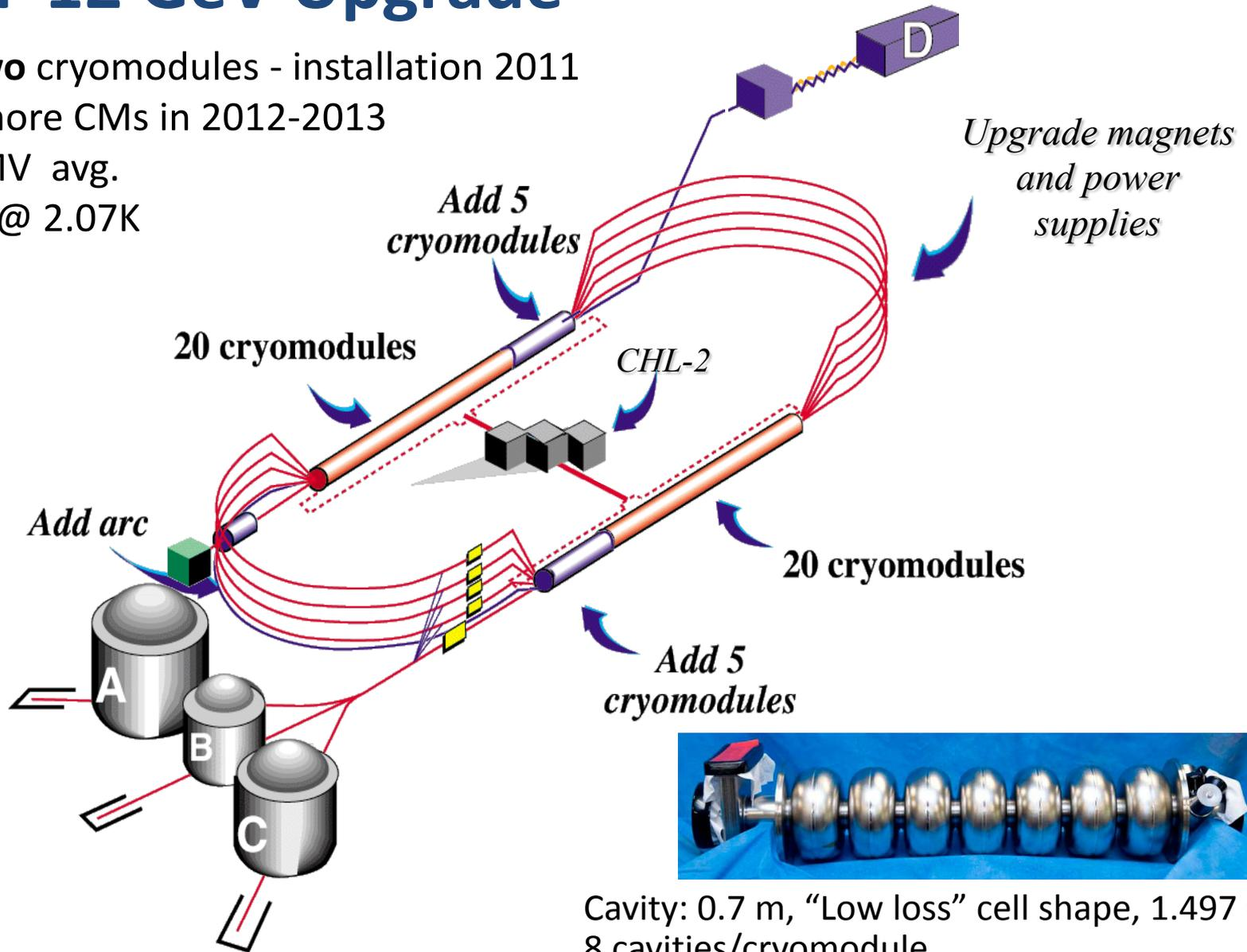
Cavity: 0.7 m, "Low loss" cell shape, 1.497 GHz
