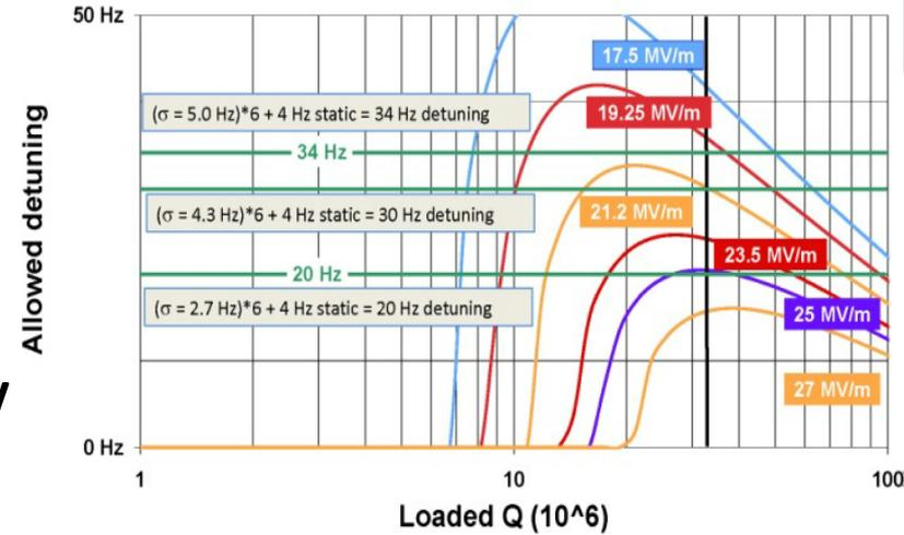
Detuning limit of C100 cavities with 12 kW of available rf power at several different operating gradients, with 460  $\mu\text{A}$  design beam current
