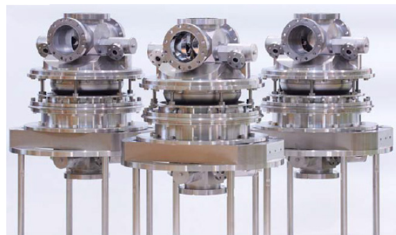
Three 2-cell cavities with 5 HOM couplers
