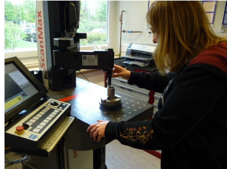
■ Equipment for tactile 3D dimension measurement
