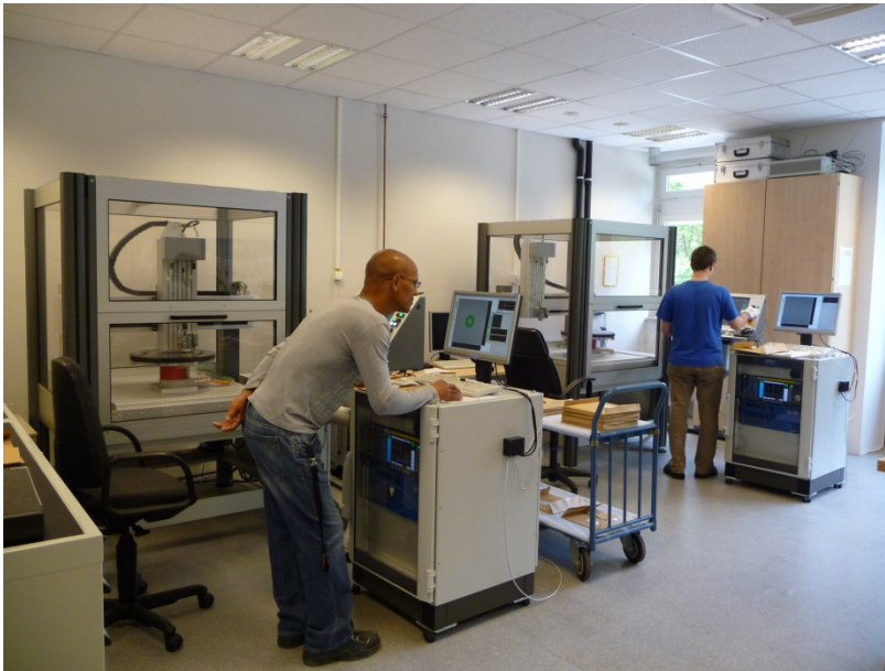
■ Eddy current scanning of XFEL niobium sheets at DESY
