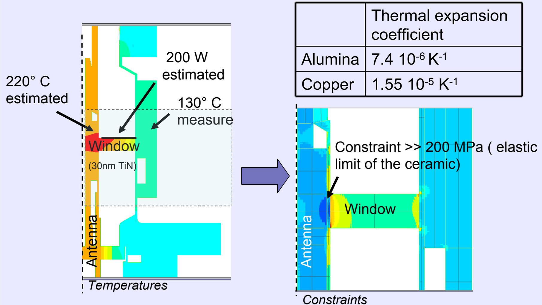
■ This very high constraint led to window's break
