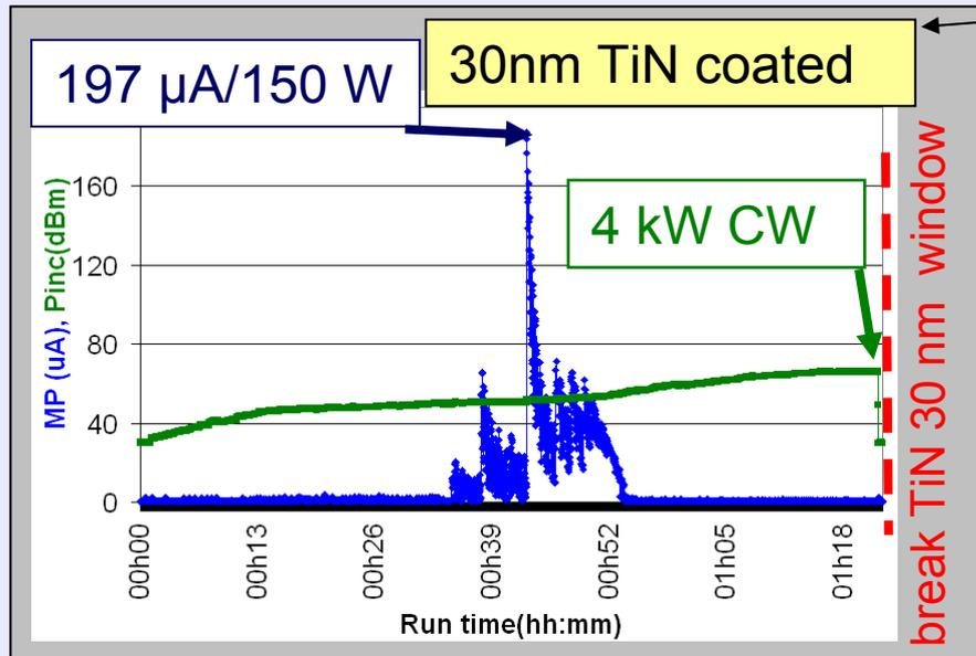
*Multipactor and power of an uncoated , a 1 nm TiN and 30 nm TiN coated window.*
