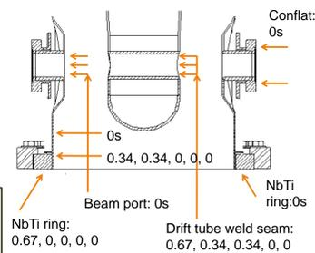
Figure 3. Surface particle counts for QWR. Particle size per in<sup>2</sup> (0.3, 0.5, 1.0, 5.0, 10.0 micron). Cleanroom background: 0s.
