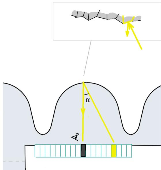
The system has 20 LED lights located at both sides of the camera aperture. We sequentially turned each of them on and off. The angle  $\alpha$  ranged from -40 to 40 degrees
