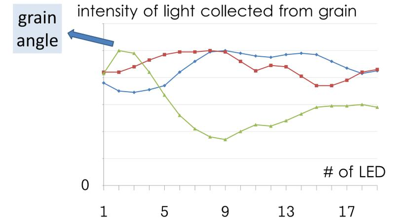
Curves for some grains have a pronounced peak. If there is a peak for some curve, we can calculate its position and, therefore, figure out the angle of the grain relative to the surface.
