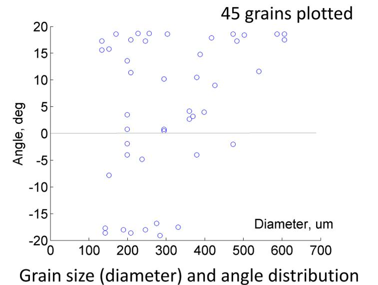
The method is a simple way to acquire information about grain angles distribution of HAZ in a cavity but is limited to estimating angles at 100-500 um scale for new and BCPed cavities (large grain, big angles)
