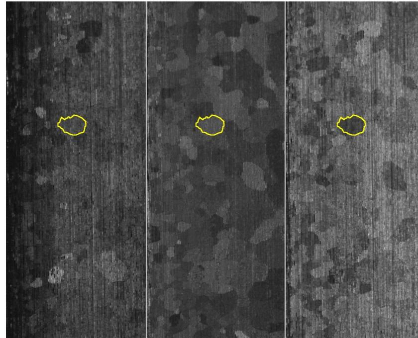
Example: snapshots for three different lights turned on. Grains have a peak in reflection at some angle (one grain is highlighted.) Vertical stripes are mechanical polishing artefacts.
