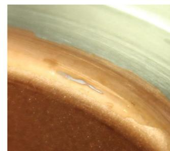
Copper removal observed near the output flange in two coupler cold sections after rf operation at FNAL.
