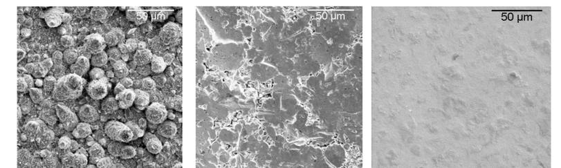
SEM photos of the copper coupon plating: (left) vendor non bead blasted, (middle) vendor bead blasted and (right) SLAC non bead blasted
