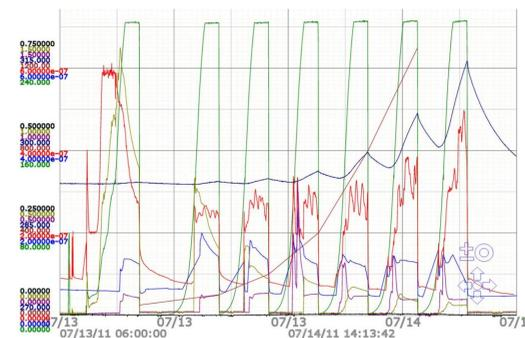
The result of room temperature rf processing of a coupler at FNAL. The green curve is the forward RF power [kW], deep blue is the coupler temperature [K], red and blue are the coupler and cavity vacuum [Torr], deep red is the rf pulse length [μs], pink and yellow are the signals from e-probes near the 4 K and 80 K flanges [mA].
