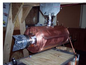
← liquid nitrogen thermal shield
