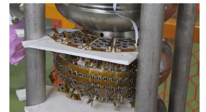
1024 T-sensors + 512 X-sensors / Cell 10 lines/cell
