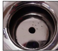
Fig. 3: Endplate after first treatment when defects appeared. Reason still unknown but maybe caused during turning of the large grain endplates.
