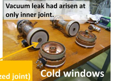
Leak point (inner brazed joint)
