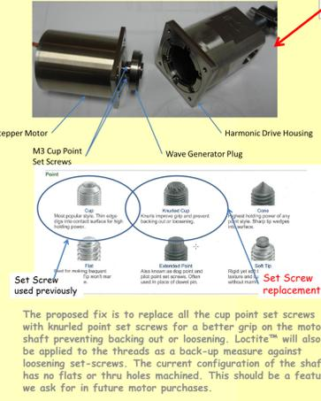
**No Slow Tuner Failure or Performance Degradation after:**
