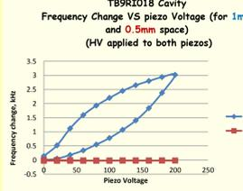
For CM2 SRF cavities tuners will be assemble with 1mm clearance. This modification will lead to modification the range of over-pressure test of CM2 at room temperature
