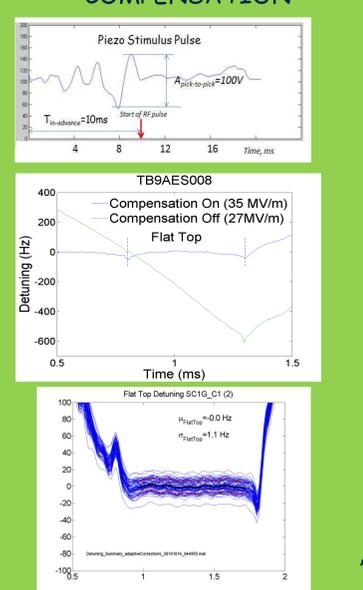
At maximum operating gradient (~35MV/M) LLRF feed-back loop OFF
