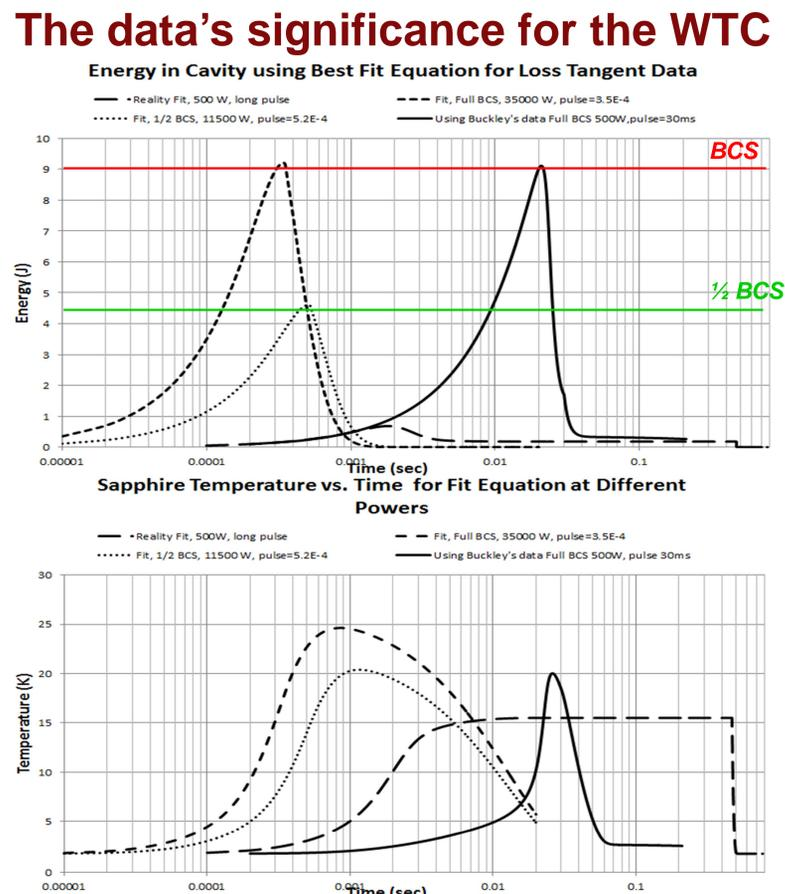
★ Top: This figure illustrates the ramifications of the STC tests. Long dashed line shows that at the maximum power that can be provided (500 W), the cavity cannot reach above 21 mT using the data acquired from the STC. However if the same results were to be achieved as those measured by calorimetry, then the cavity would respond as designed with 500W of power, as the solid line shows.
