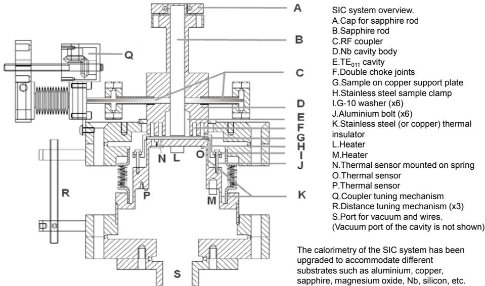
The calorimetry of the SIC system has been upgraded to accommodate different substrates such as aluminium, copper, sapphire, magnesium oxide, Nb, silicon, etc.
