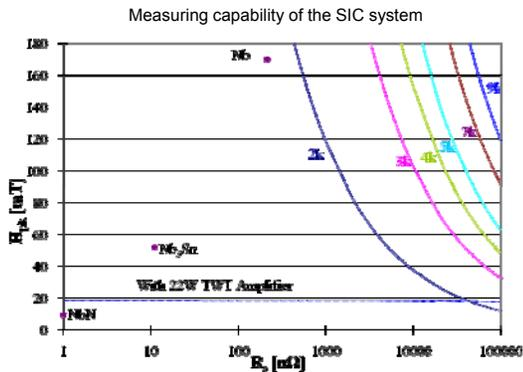
$$\text{Surface Impedance } Z_s = \frac{P_{rf}}{kH_{pk}^2} + i\omega\mu_0\left(\lambda_{ref} + \frac{f - f_{ref}}{M}\right) \quad \text{with } k = 3.70 \times 10^7 \left[ \frac{W}{\Omega T^2} \right] \quad M = 20.5 \text{ Hz/nm} \quad \frac{H_{pk}}{\sqrt{J}} = 0.354 \left[ \frac{T}{\sqrt{J}} \right]$$
