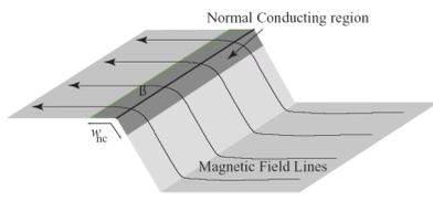
Geometrical enhancement, contamination, etc., creates a region with suppressed superconducting critical field, at field greater than  $H_c/\beta$  the region quenches and the power dissipation increases unstably.
