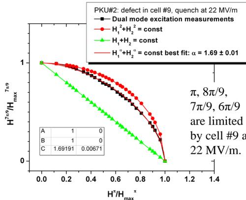
PKU2: defect in cell #9, quench at 22 MV/m
