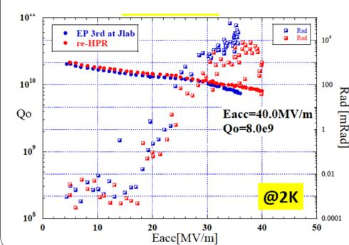
The left figure shows the ICHIRO#7's results which were tested in Jlab. All preparations including EP were done in Jlab. In this case, X-ray onset is around 15MV/m. ICHIRO#7 has a lower X-ray onset and much serious in amount compared with ILC TESLA shaped cavities treated and tested in Jlab. ICHIRO cavity shape has a few higher Ep/Eacc ratio: 2.3 with ICHIRO 9-cell and 2.0 with TESLA 9-cell. Is the difference of cell shape related to this result?
