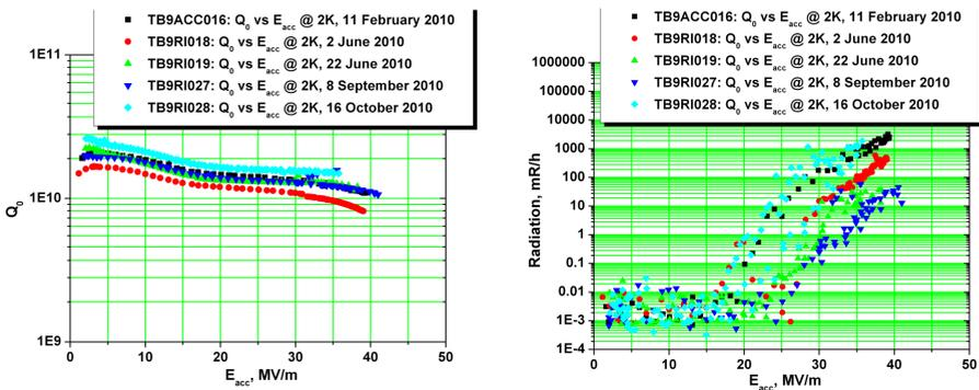
Five cavities from Research Instruments have been tested as part of ILC yield in 2010. All five cavities have met ILC specifications after the second pass. In many test advanced instrumentation such as thermometry and OSTs have been used to study performance and limitation of the cavities.
