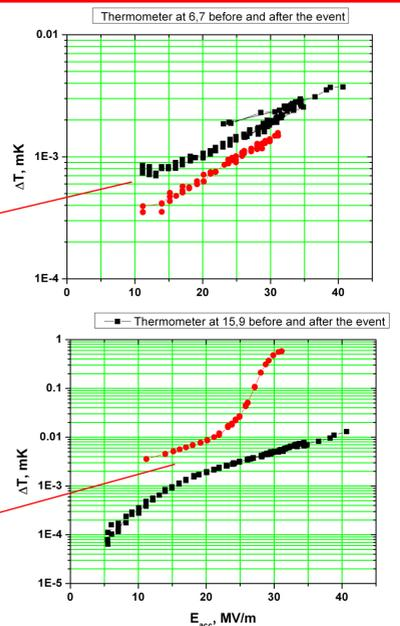
The data above shows heating field dependence change before and after FE event at the original quench location and new quench location. The change in  $T$  vs  $E_{acc}$  for the original quench location suggest that niobium surface modification is involved in sudden FE event.
