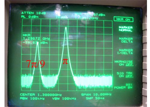
Mode mixing was observed for  $\pi$ ,  $4\pi/9$ , and  $2\pi/9$  modes measurements.  $4\pi/9$  mode mixed with  $3\pi/9$ ,  $5\pi/9$ , and  $2\pi/9$  mode mixed with  $\pi/9$  and  $3\pi/9$ .
