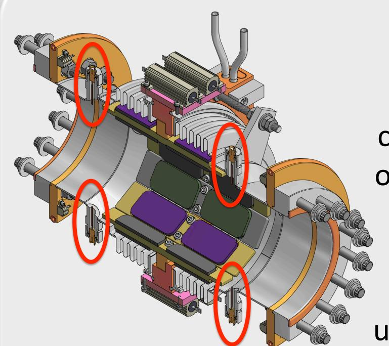
The HOM loads absorb power in RF-lossy absorber tiles. HOM spectra were obtained by connecting a spectrum analyzer to one of 8 RF pickups and measuring incident power over frequencies from 0-50 GHz. A typical scan requires several minutes of uniform beam and has a resolution of approximately 50 kHz.
