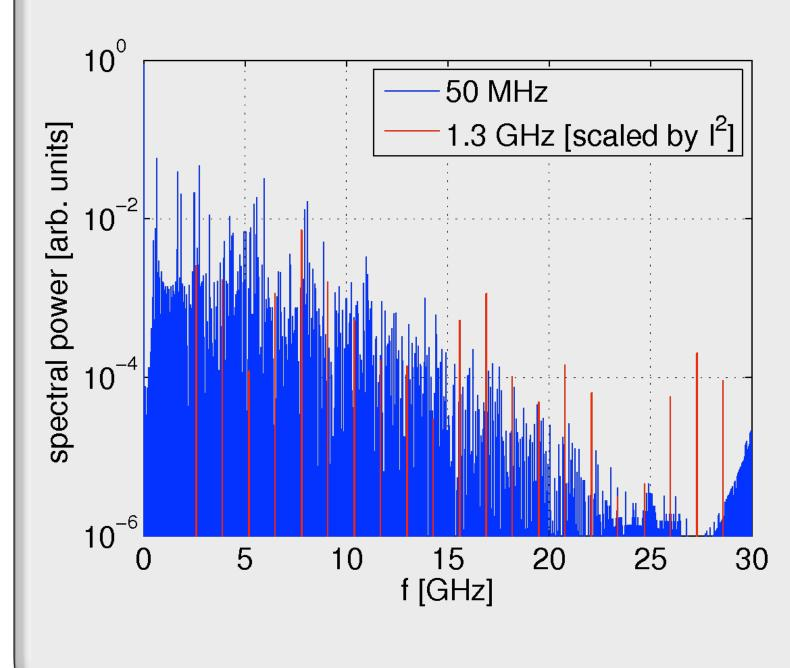
When the bunch repetition rate  $f_{rep}$  is also changed, the HOM spectra should vary with  $I^2/f_{rep}$ . At high frequencies, the  $f_{rep}$ =1.3 GHz spectrum has strong spectral lines out much further. This suggests that the bunch length decreased in the weeks between the 50 MHz measurement and the 1.3 GHz measurement.
