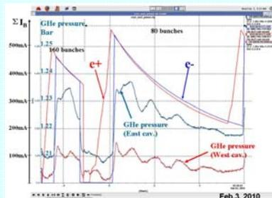
GHe pressure of East cryostat are nearly same at 80 and 160 bunches
