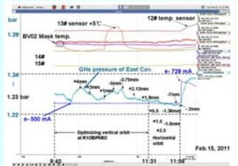
GHe pressure is optimized by beam orbit within 1.26bar that is a interlock threshold. The maximum e- current reached 825mA in test
