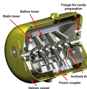
Figure 1: Design of the sc 325 MHz CH cavity for the GSI UNILAC upgrade.
