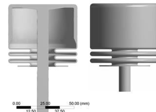
Figure 3: Schematic overview of a dynamic bellow tuner.
