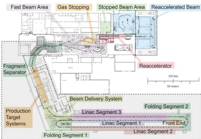
Layout of the FRIB facility displaying the folded linac design, 400 kW CW production target, fragment separator, as well as nuclear science experimental facilities for fast, stopped, and re-accelerated radioactive beams.
