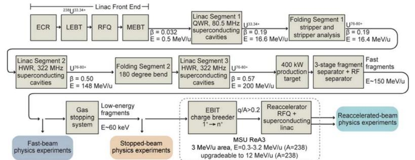
Functional System Diagram of the FRIB Facility
