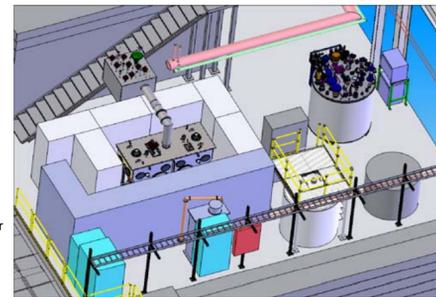
FRIB is currently assembling a Technology Demonstration Cryomodule (TDCM) with two β = 0.53 half wave resonators and one 9 T solenoid. The TDCM serves as half-wave cryomodule prototype as well as 2K systems test.
