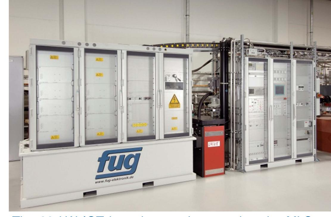
The 80 kW IOT based transmitter used at the MLS. This transmitter is used as prototype for the klystron-based 270 kW transmitters for the injector cavites at B*ERL*inPro.
