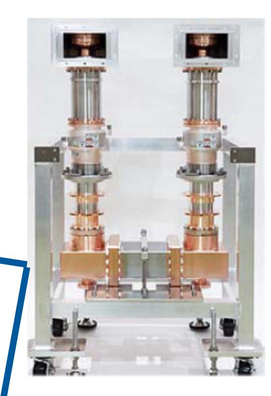
cERL fundamental power couplers on the coupler test stand. They are the candidates to be used at the photo injector and the booster cavities
