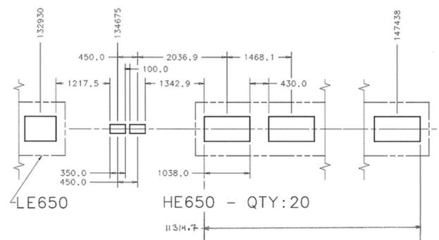
Figure 2. 650 MHz beta = 0.9 cryomodule (HE650) lattice spacing [3]. Dimensions, in mm, are effective RF and magnetic field lengths, which for cavities is approximately end iris to end iris distance. HE650 refers to the 20 beta = 0.9 cryomodules. Large rectangles represent RF cavities.
