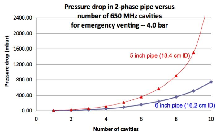
Figure 4. Loss of cavity vacuum to air — venting pressure drop in 2-phase pipe (differential pressure)
