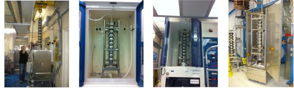
Field flatness check, Ultrasonic, flash BCP, HPR, Assemble, Baking at JLAB
