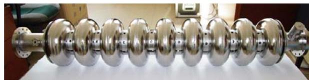
Figure 1: Picture of 9-cell LG cavity PKU2 [5].
