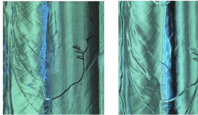
Figure 7: Typical sharp grain-boundary in AC158 after BCP treatment (left), same location after EP with smoothed grain boundary (right).
