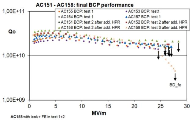
Figure 5:  $Q_0(E)$ -performance after BCP treatment, measured at 2K. All cavities limited by thermal-breakdown; AC158 with strong FE [13].
