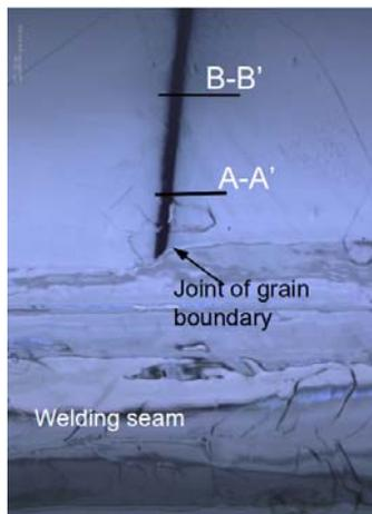
Figure 2: Optical inspection picture of PKU-LG1. B-B' indicates the location of the profile scan in Figure 3 [10].
