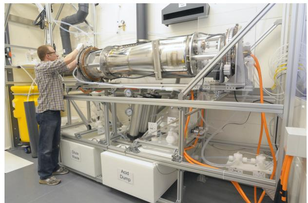
Figure 2: Prototype QWR installed in the new EP tool.
