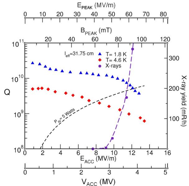
Figure 6: Results of prototype QWR cold test.
