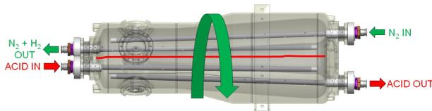
Figure 5: Diagram of the acid/N<sub>2</sub> flow. The red line represents the level of the acid bath inside the cavity.
