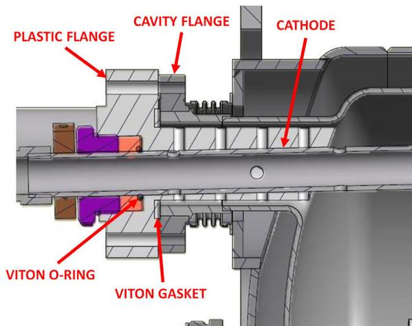
Figure 3: Precision plastic flange for cathode loading and proper alignment inside of cavity rf space.
