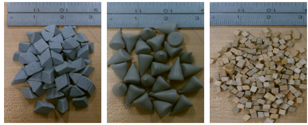
Figure 2: Picture of some of the media used for CBP of cavities at Fermilab to achieve a mirror like finish on the inside of cavities.
