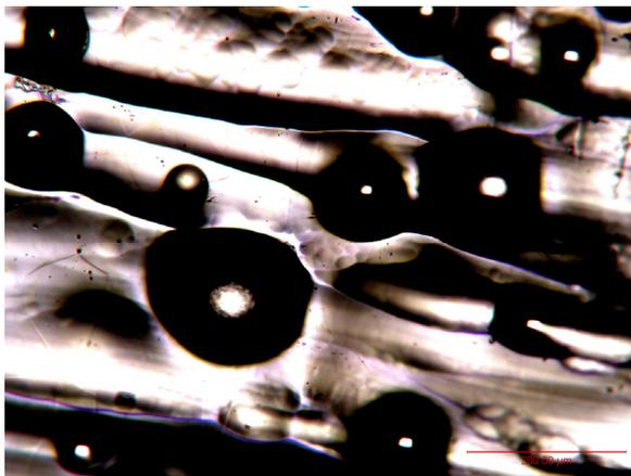
Fig. 7: Pits formed at the downward facing surface of a flag electrode.
