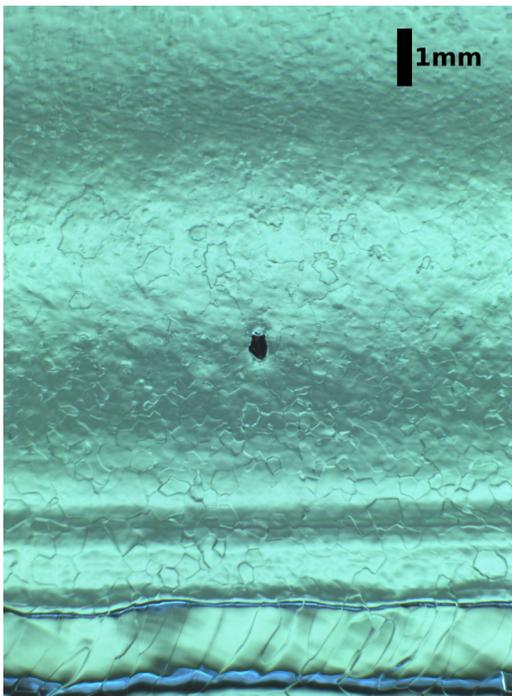
Figure 5: Inner cavity surface of the spot marked in Fig. 4. At the bottom of the picture the welding seam of the equator can be seen.
