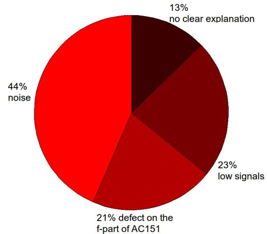
Figure 7: Categories for failing second sound quench location measurement.
