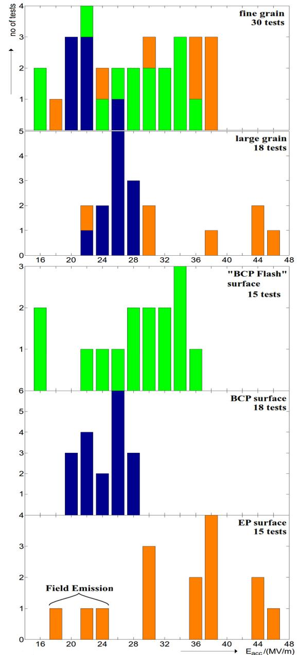
Figure 2: Gradient performance of cavities tested by material and surface treatment – the colors indicate the surface treatment.
