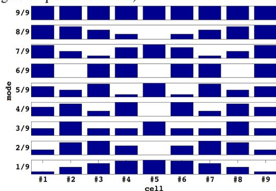
Figure 3: Field distribution in a 9-cell cavity for all fundamental modes, normalised to the max. field in each mode.
