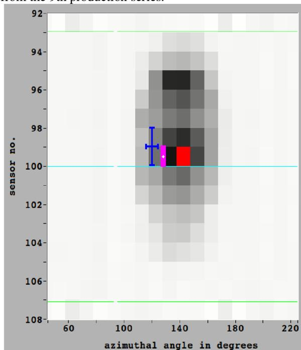
Figure 4: Section of the temperature map of Z161 in  $\pi$ -mode. Cell 2 is visible in an angular range from 45° to 225°. The turquoise line shows the position of the equator.
