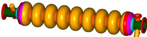
Figure 1: 3D model of a 9-cell 1.3 GHz European XFEL design cavity.
