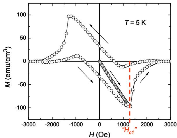
Figure 2: Complete magnetization loop indicating gradient performance potential conducted at 5 K,  $H_{c1}$  (i.e., field of first significant flux penetration)  $\sim 1300$  Oe, and  $H_{c2}$  at high field  $\sim 2750$  Oe.
