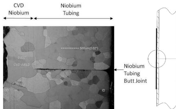
Figure 3: Cross-sectional optical micrograph of CVD-welded tensile butt-joint test specimen (left) and schematic showing orientation (right) of butted niobium tubes with  $\sim 0.03$ " thick CVD niobium. Measured ultimate tensile strength was 39.327 ksi vs. reported strength of pure annealed niobium of 43.5 ksi.
