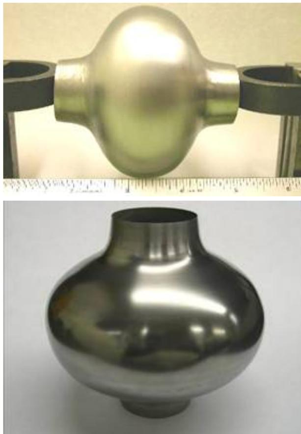
Figure 1: Freestanding seamless CVD niobium cavity prototype fabricated by Ultramet.
