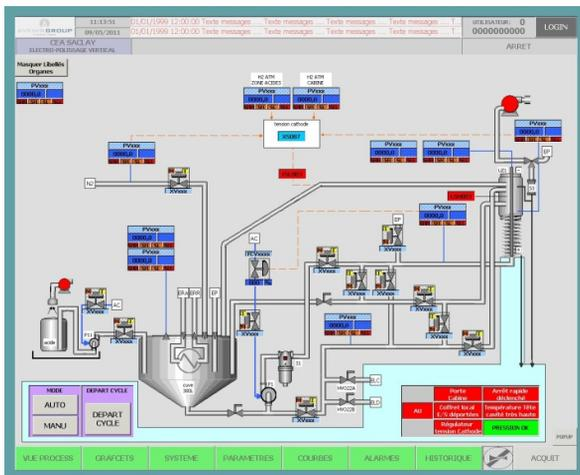
Figure 2: Flowsheet of the process displayed on the touchscreen.
