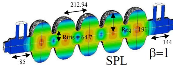
Figure 6: 704 MHz SPL cavity to be electro-polished in VEP set-up.
