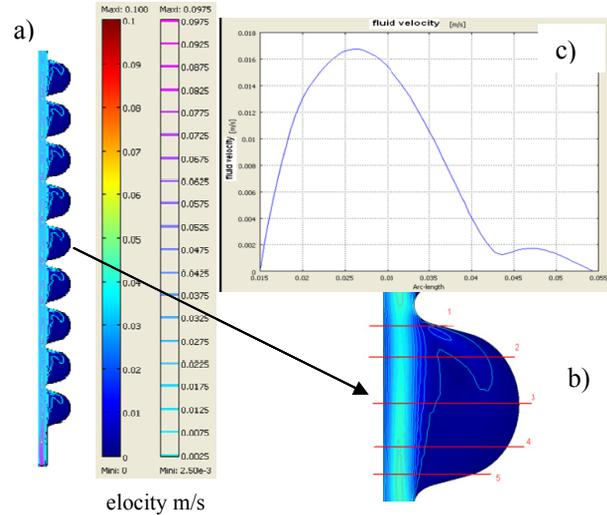
Figure 4: a) Fluid modeling in the ILC cavity for  $v_{max}=0.2\text{m/s}$ . b) Zoom of the central cell. c) For each line (1 to 5), the distribution profile between the cathode and the cavity is similar.
