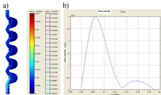
Figure 8: a) Fluid distribution in the 5cell SPL cavity and b) fluid velocity profile along the red line. Shaped cathode makes it possible to increase fluid velocity in the cell.
