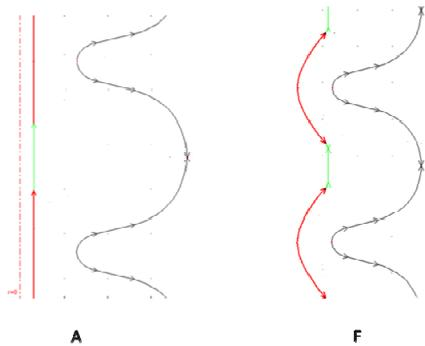
Figure 11: Alternative insulated cathode shapes numerically tested for the SPL cavity. At the cavity:  $V=15V$ , at the cathode.  $V=0$ . Insulated parts of the cathode are in red.
