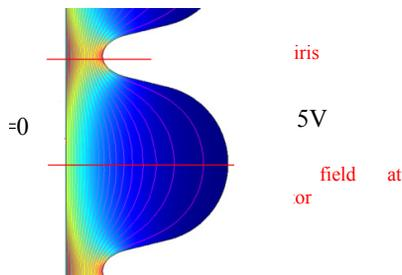
Figure 9: Potential distribution in a Tesla shape cell using a cylindrical cathode. At the Cathode,  $V=0$  and at the anode,  $V=15V$ .
