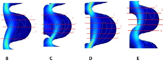
Figure 5: Shapes tested to improve fluid distribution inside the cells.
