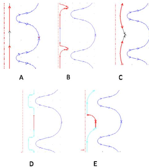
Figure 10: Alternative insulated cathode shapes numerically tested for the Tesla cavity. At the cavity:  $V=15V$ , at the cathode:  $V=0$ . Insulated parts of the cathode are in red (A, B, C) and in light blue (D and E).
