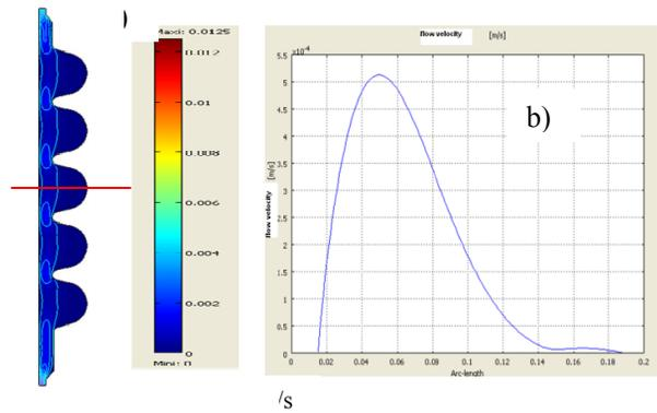
Figure 7: a) Fluid distribution in the 5cell SPL cavity and b) fluid velocity profile along the red line.
