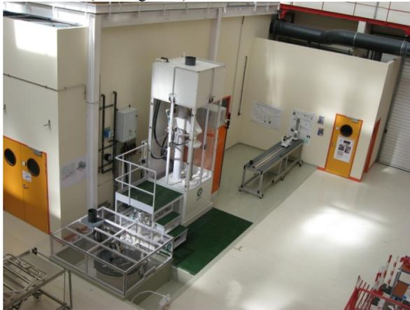
Figure 1: VEP set-up at CEA Saclay. 1: Main cabinet for cavity treatment. 2: Acid tank located in a pit. 3: Table for assembly prior to VEP.
