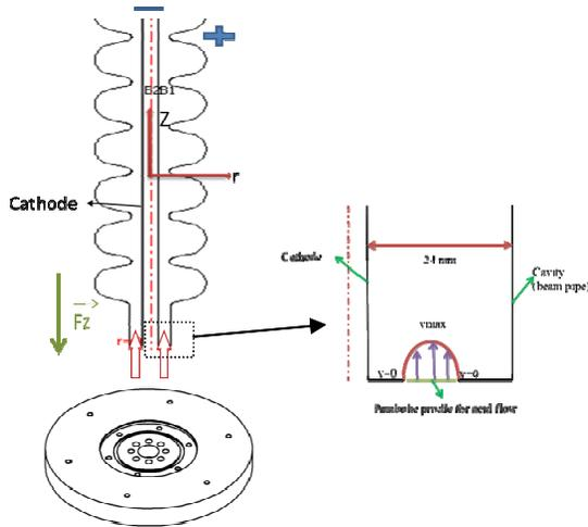
Figure 3: 2D axi-symmetry used for modeling of VEP. We have considered a crown of fluid entering the cavity with a parabolic profile.
