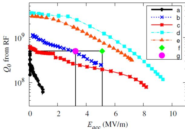
Figure 3: RF performance at 4.3 K of a single cavity (SC246) as it progresses through the R&D leading to the refurbishment. The green diamond (f) indicates the original 4.5 K FRIB goal. The purple circle (g) indicates the 4.5 K ReA3 goal. The curves (a-e) are explained in the text.
