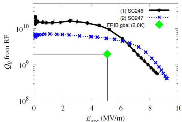
Figure 6: RF tests at 2 K on two refurbished QWRs immersed in a helium bath. The green diamond indicates the FRIB 2 K design goal. Note that  $E_{peak}/E_{acc} = 6.16$ , and  $B_{peak}/E_{acc} = 13.9$  mT/(MV/m).
