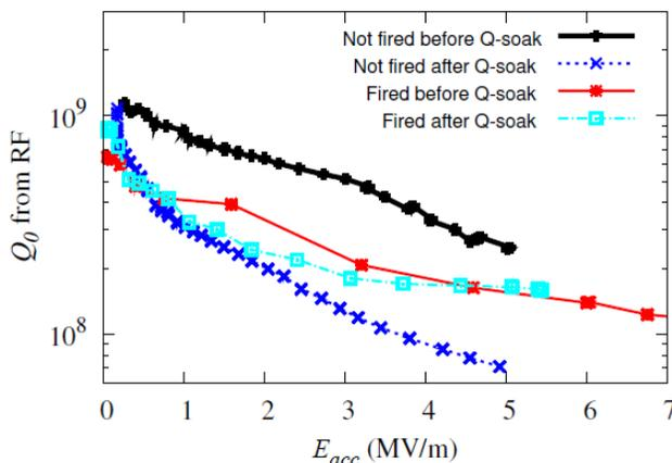
Figure 4: RF measurements before and after a 10 hour “ $Q$  disease soak” at 100 K. The RF measurements were performed with immersion in a 4.3 K helium bath.
