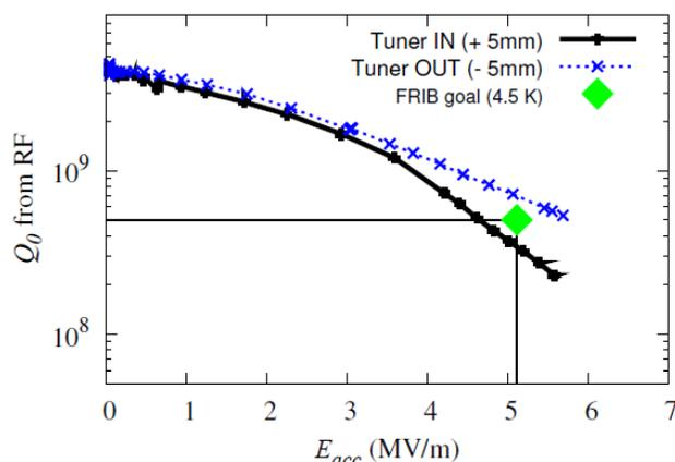
Figure 2: Initial test results at 4.3 K for the second production QWR (SC247) prior to helium vessel welding.
