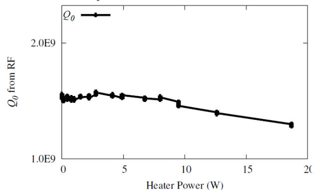
Figure 5: RF measurements with a heater on the tuning plate, with the cavity immersed in a 4.3 K helium bath.
