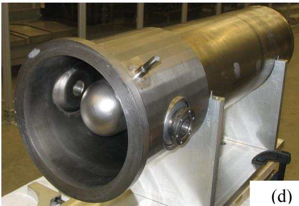
Figure 1: Design evolution of the ReA3 QWR: (a) original RIA QWR prototype; (b) ReA3 production QWR; (c) planned refurbishments for ReA3 (under development); (d) photograph of ReA3 production QWR.
