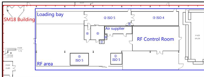
Figure 3: SM18 top view, delimited in blue the new cleanroom space as proposed in the last refurbishment plan (①softwall cleanroom, ②preparing area, ③assembling room, ④personal access, ⑤air shower, ⑥cleaning and rinsing space, ⑦ultra pure water production, ⑧high pressure rinsing, ⑨softwall cleanroom).
