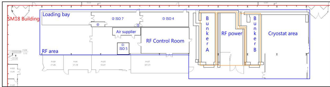
Figure 2: RF area within the SM18 building (①softwall cleanroom, ②preparing area, ③assembling room, ④personal access, ⑤air shower).
