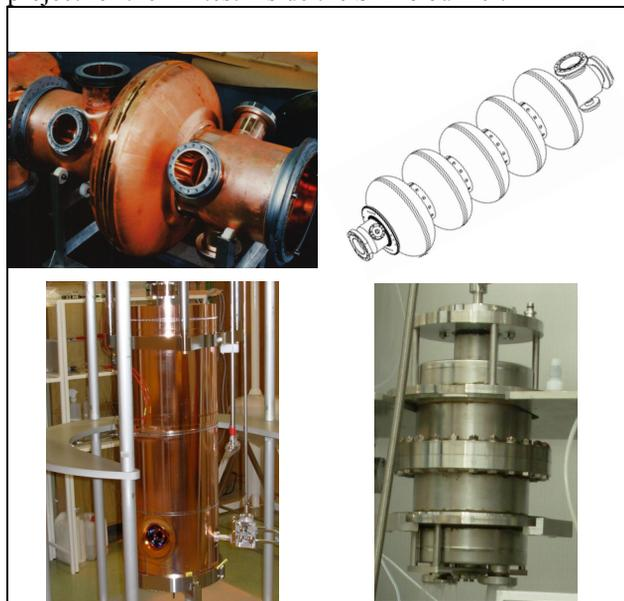
Figure 1: LHC cavity (top left), SPL cavity (top right), HIE Isolde cavity (bottom left), and quadrupole resonator (bottom right).
