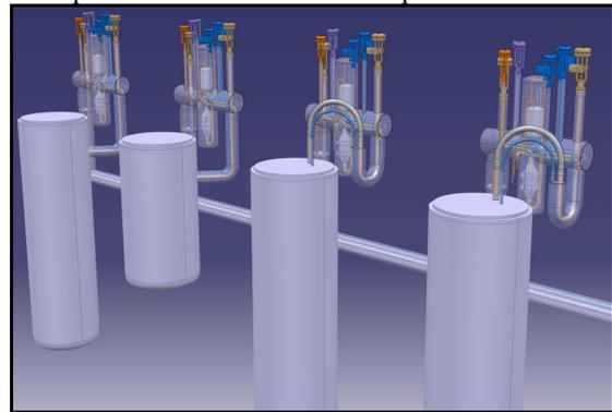
Figure 6: new design of the cryostat-cryoline interfaces around the vertical cryostats (two on the left for 2 K operation, two on the right for 4.5 K operation).
